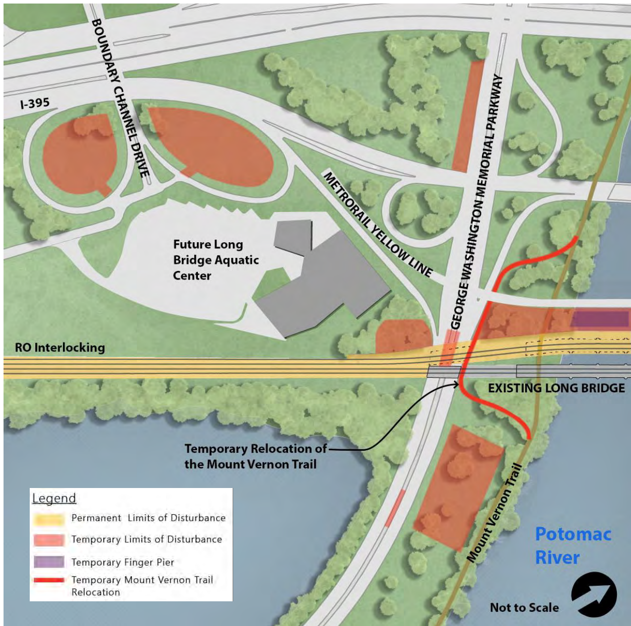
Figure 6-2 | Construction Staging and Access in the Vicinity of the George Washington Memorial Parkway
