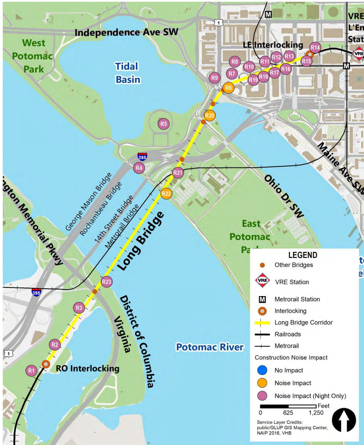
Figure 10-7 | Construction Noise and Vibration Impact Assessment Results
