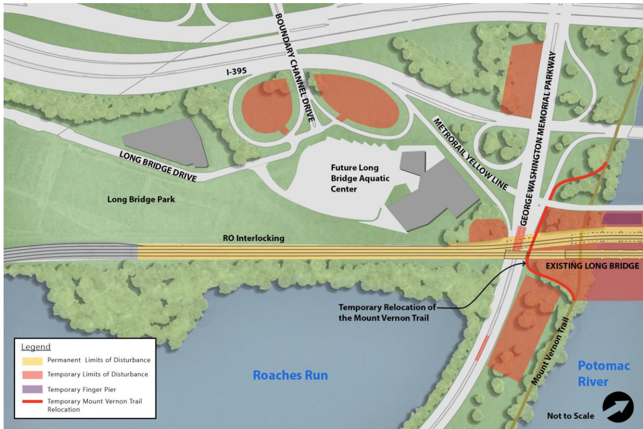
765 Figure 3-20 | Action Alternative B Construction Access and Staging Locations – RO Interlocking to 766 Potomac River
