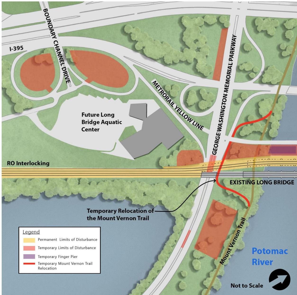
622 Figure 9-6 | Mount Vernon Trail Rerouting during Construction
