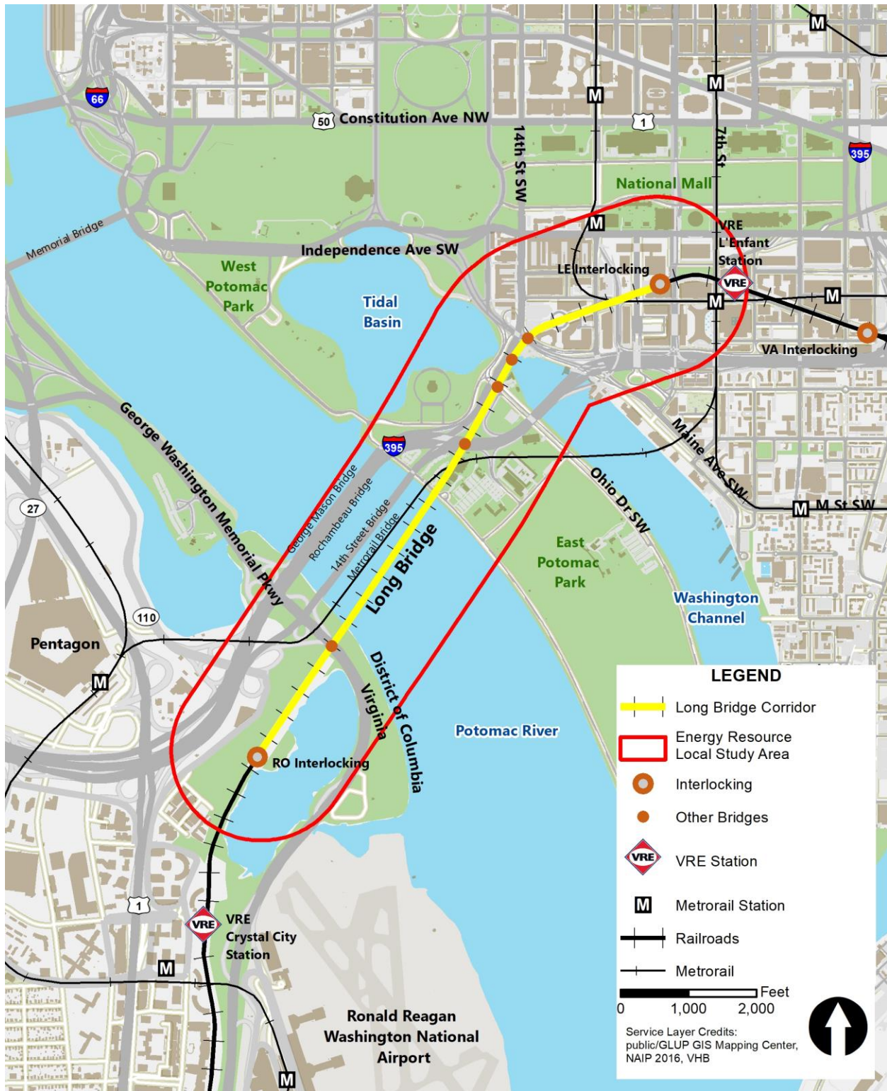
60 Figure 11-1 | Local Study Area for Energy Resources
