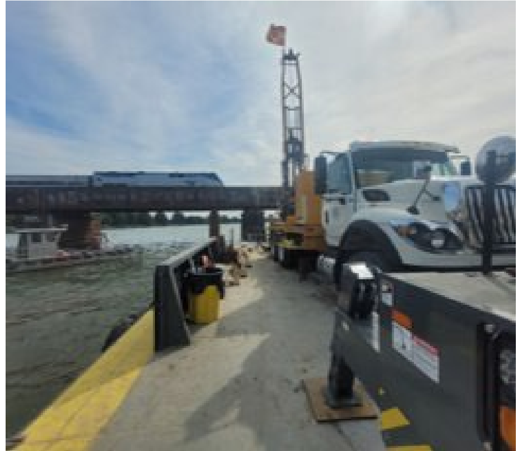
Soil Boring Sampling in Potomac River
