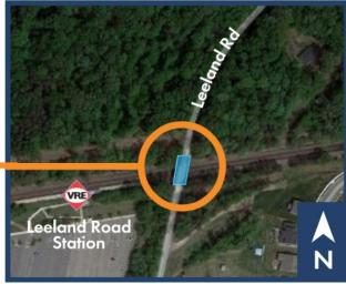
This project will increase the horizontal and vertical clearance of the roadway bridge to allow for the third track and a potential future fourth track.
