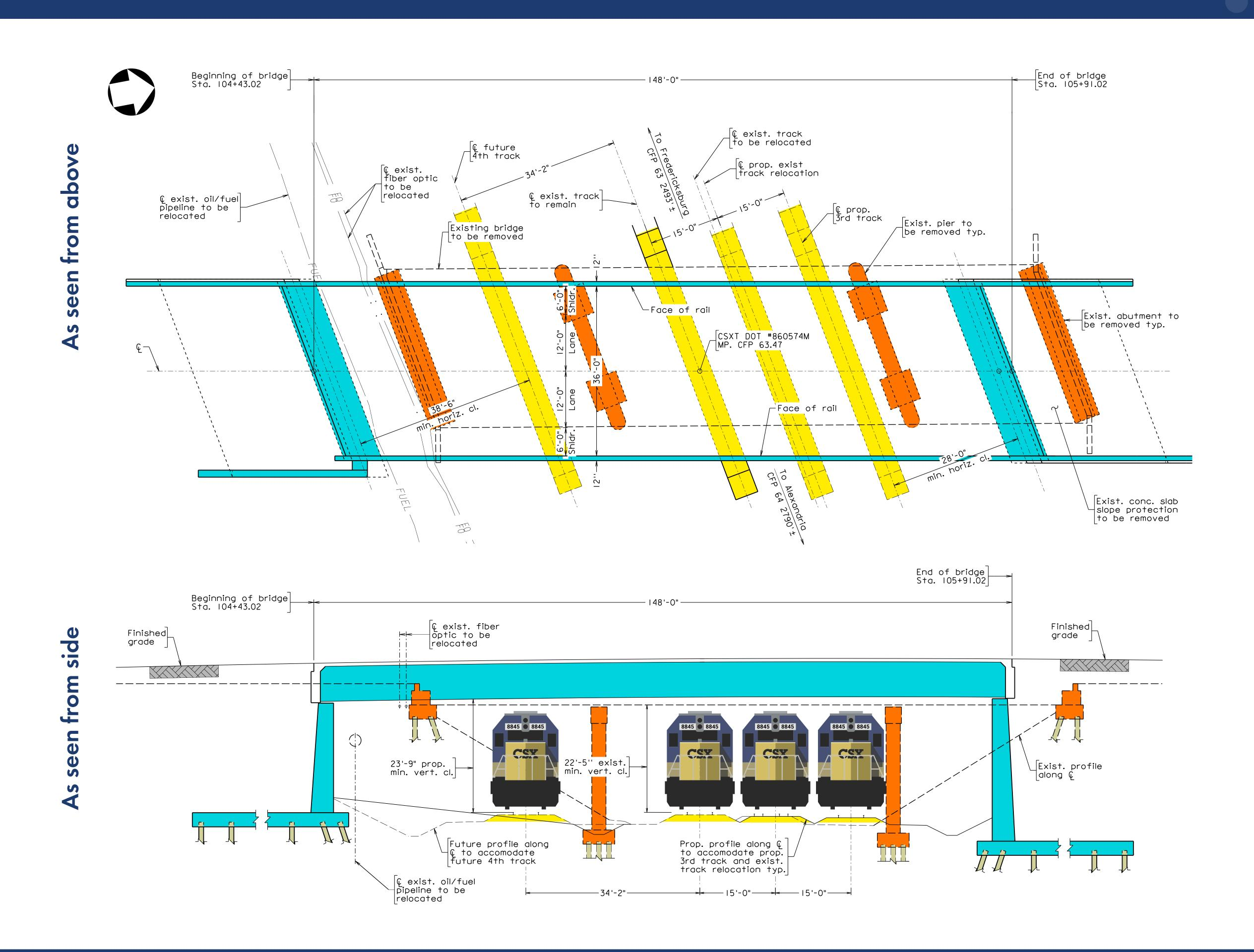
These plans show the current and proposed Leeland Road Overpass bridge. This project will increase the height and width clearance of the bridge to allow for construction of a third track underneath.
